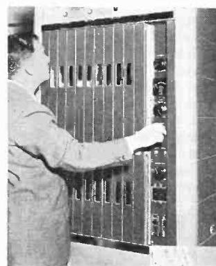
New, easy-to-reach vertical control panel. Just slide front door to left 4 inches (to automatic stop point). Transmitter interior not accessible until door is moved further left beyond this stop position — when interlocks and grounding switches function.
