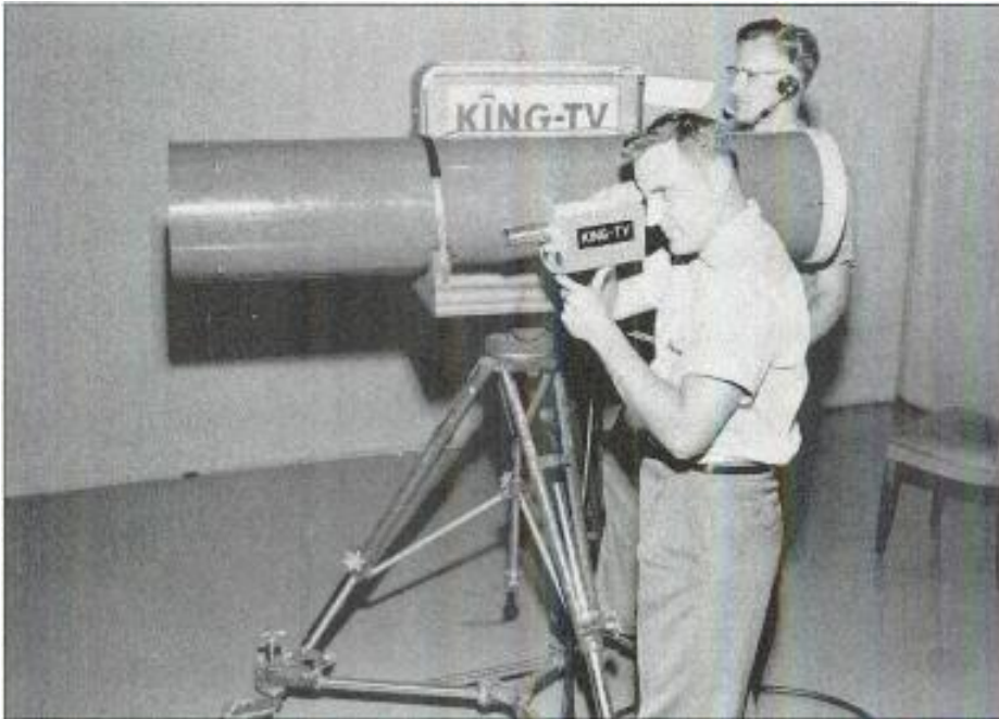
In 1951, KING-TV engineers Earl Thoms (in foreground) and Al Smith (in back) developed and produced the nation's first 100-inch camera lens, designed to capture close-ups of the hydroplane races. The lens was loaned to the networks when similar shots were called for.
