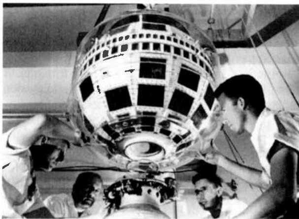
Technicians attaching the Telstar satellite to a Delta rocket for launch. Property of AT&T Archives. Reprinted with permission of AT&T
