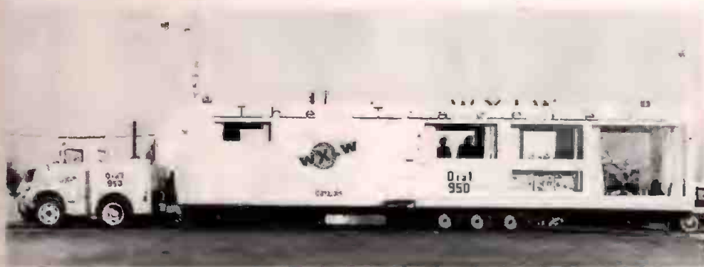
ROLLING RADIO STATION now in operation for WXLW Indianapolis, "The Traveler," is a "self-sustaining" unit, according to the station. Statistics: 45 feet long, 8 feet wide, more than 12 feet high. It carries a 10,000 watt-producing gasoline generator, 250 gallons of fresh water. It has a studio, a control room, a bath, a shop area, a lounge and storage areas.
