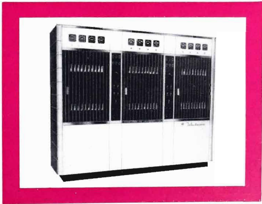
1-KW TYPE TTU-1B (FOR ERP* TO 27 KW). This transmitter and a UHF Pylon Antenna, can develop from 24 to 27 kw ERP on any channel, 14 to 83. TTU-1B is self-contained and air-cooled. It is well suited as a driver for a high-power amplifier.
