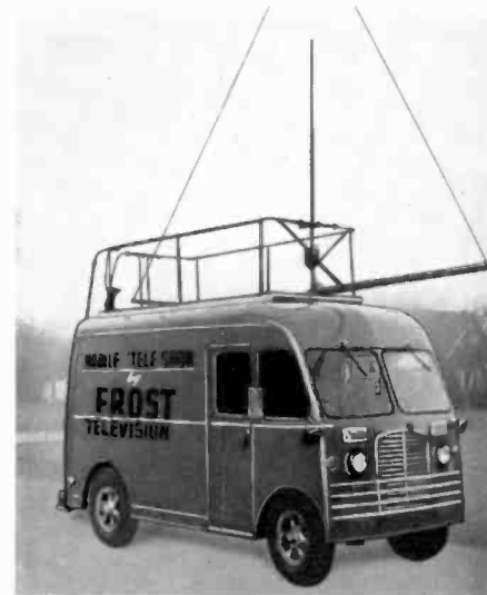
"Mobile Teleshov" van houses one console and two table models, has a collapsible antenna which is completely rotatable. Truck can seat ten people.
