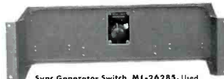
Sync Generator Switch, MI-26285. Used to switch outputs of either of two sync generators over to studio equipment. One selector for all 5 signals (horizontal, vertical, blanking, sync, and CRO sync).
