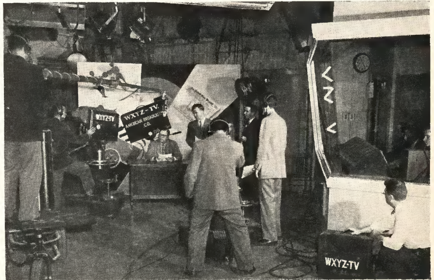
WXYZ-TV's smaller studio, with fluorescent banks and incandescent spots for lighting, is equipped with two RCA studio cameras on pedestal dollies, and a third camera for stand-by, shown in lower right. Row of monitors appearing on the right, inside control room, is as in sketch, page 21.
