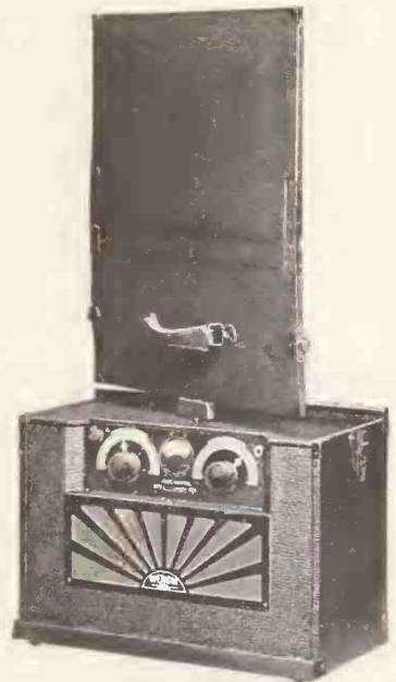
The 1925 Operadio removed from cabinet and ready for use. The cover is the aerial; the case may be closed and carried like a piece of hand luggage.
