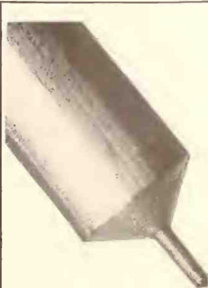
The point of a Sonora semi-permanent needle magnified many times after having played a number of records. Note the uniform shaft—a great saver of records.
