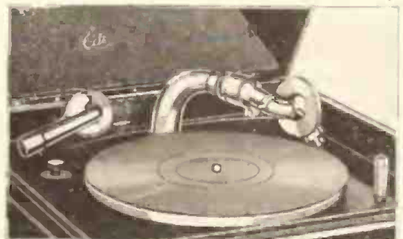
Showing back view of needle equipment in position for playing lateral cut records.
