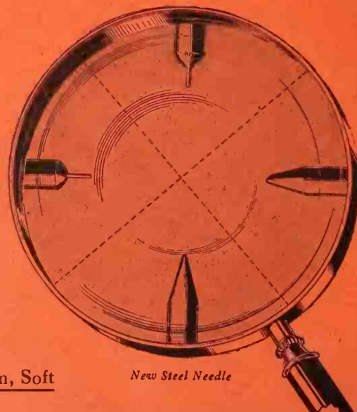
Sonora Semi-Permanent Silvered Needle After Being Used Fifty Times
