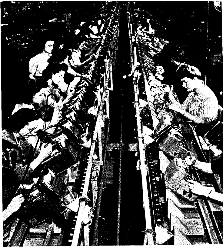
Assembling automobile radios as they move along the conveyor belts of the RCA Victor plant at Indianapolis, Ind.
