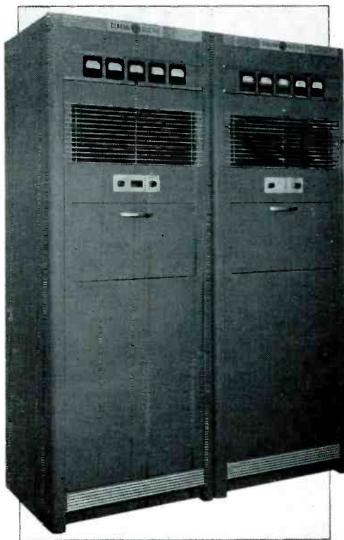
FIG. 7. COMPLETE G.E. 1-KW. TRANSMITTER REQUIRES LESS THAN 10 SQ. FT. FLOOR SPACE
