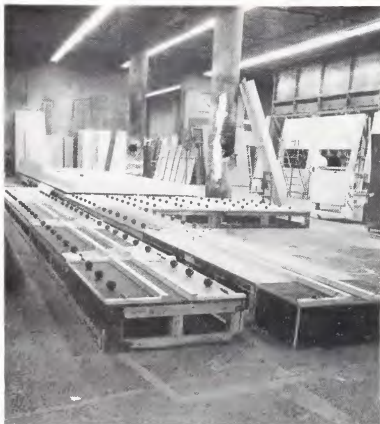
The "gimmick" to re-create the joggle of train in motion was strung-together series of lacrosse balls. Original idea was hatched for CBC-TV show "The Serial" by the show's designer, Harry Maxfield.
