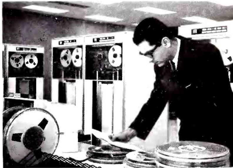
7. Next, data is fed to IBM 1401 tape computer for print-out of competitive data and storage for future tabulations. BAR vice president and general manager, Joe Rosenberg examines a day's machine run
