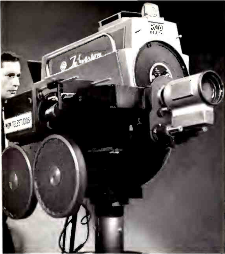
"GEMINI"—is the name of this twin camera system, employing a TK-60 Studio Camera which shares its lens with a 16mm film camera adjacently mounted. The operator uses the viewfinder of the television camera just as if he were shooting with the TK-60 alone. Final product, a high quality television tape and a high quality 16mm film duplicate, eliminates the problem of the kine-scope as a factor in spot use of taped commercials and programs. Exclusive rights to "Gemini" are held by MGM.
