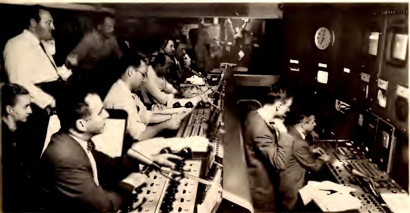
The most "gainfully" employed man in the control room at a network studio in New York, audio control engineer (left foreground) keeps sound variations between limits ("riding the gain") via knobs (pots) on audio console. He mixes, fades, etc., with one eye on volume indicator on vertical panel
