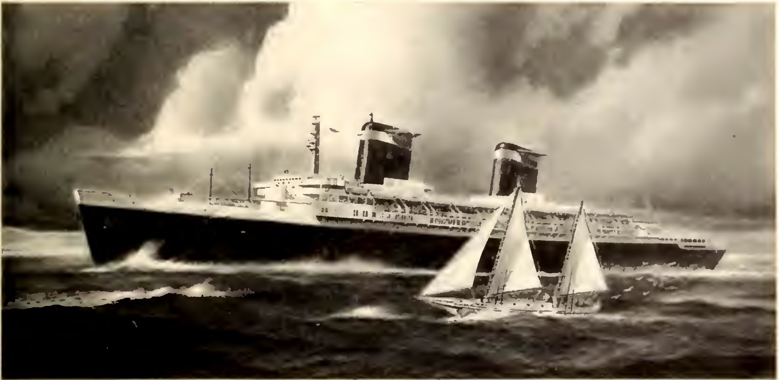
S. S. "United States". Built at Newport News, Virginia. Fastest, most modern passenger ship ever built in this country. Length, 990 feet. Beam, 101 feet. 175 feet from keelson to funnel-top. Cost, over $70,000,000.00.
