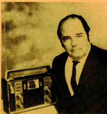
Dr. T. L. Wadley with the Barlow-Wadley XCR-30, which he designed. With the British-made Racal receivers, the XCR-30 was the first of a new breed of communications receivers. The Wadley circuitry permits tuning the full shortwave spectrum without mechanically switching bands.
