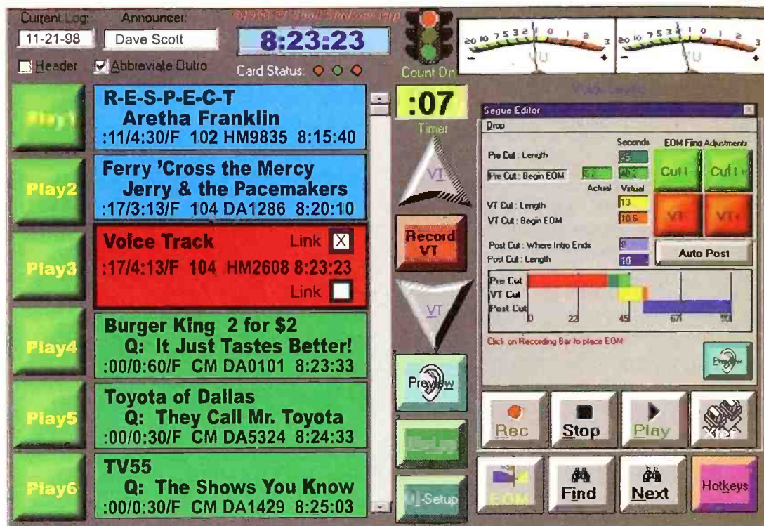
Here's Scott's Voice Trax Via Internet (VTVI) software, shown with the optional Segue Editor. VTVI allows a distant announcer to pre-record a 4 hour show in about 15-20 minutes with nothing more than a Windows computer, an Internet connection and a good microphone.
