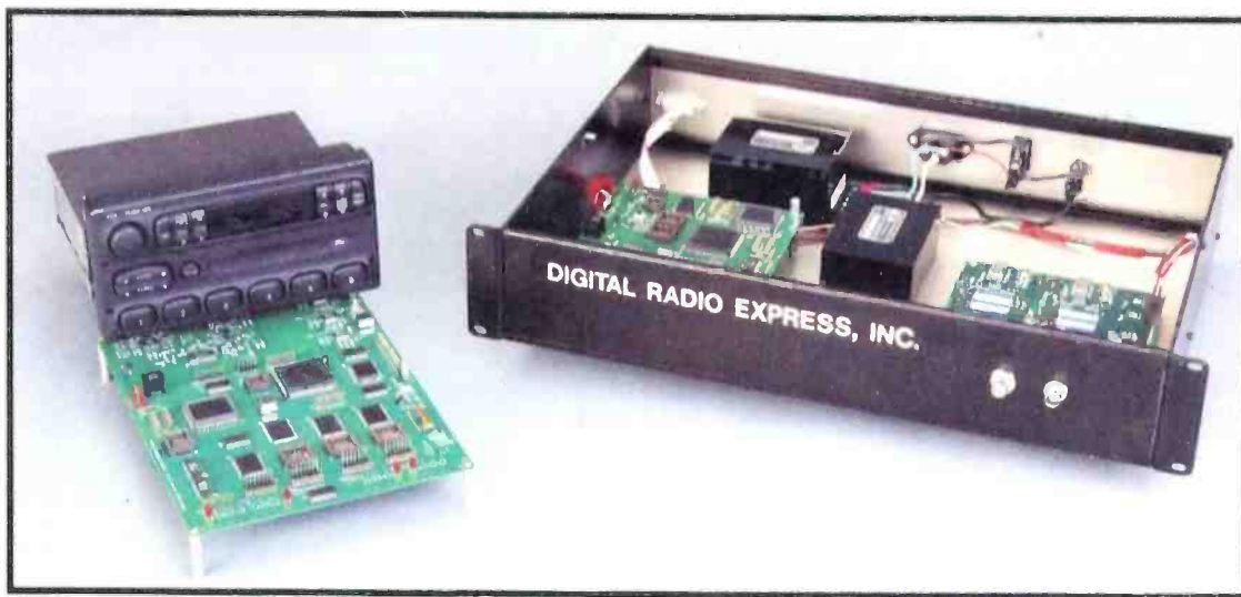
DRE's receiver, linked to a Ford factory stereo; DRE's IBOC exciter. Source: DRE
