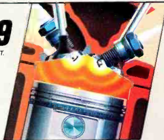
The NAPS-Z engine with 2 spark plugs per cylinder burns fuel more efficiently.
