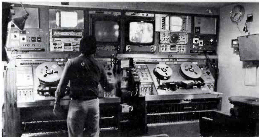
Feeds of news stories from satellites and from NBC bureaus are monitored and recorded here using RCA TK-70 two-inch quad VTRs.
