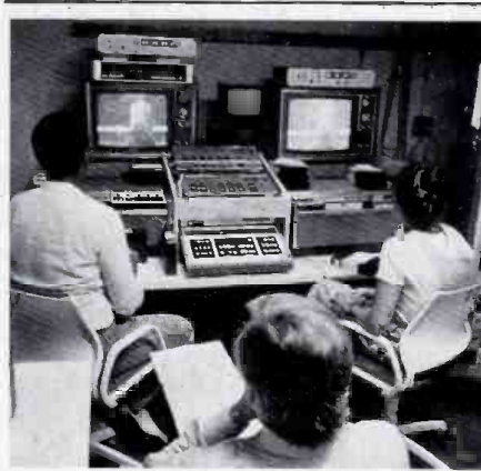
An "E.J." (Electronic Journalism) editing room at NBC News. Weekend Sports Director Dick Schaap supervises the editing of a sports piece on Sony 3/4" BVU 200 editing machines.
