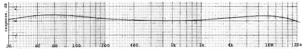
Figure 4 KEX Transmitter, Westinghouse 50-HG-1, 50 kw Modulation Response, 50 Per Cent Modulation taken at Plate Tank Sample.
