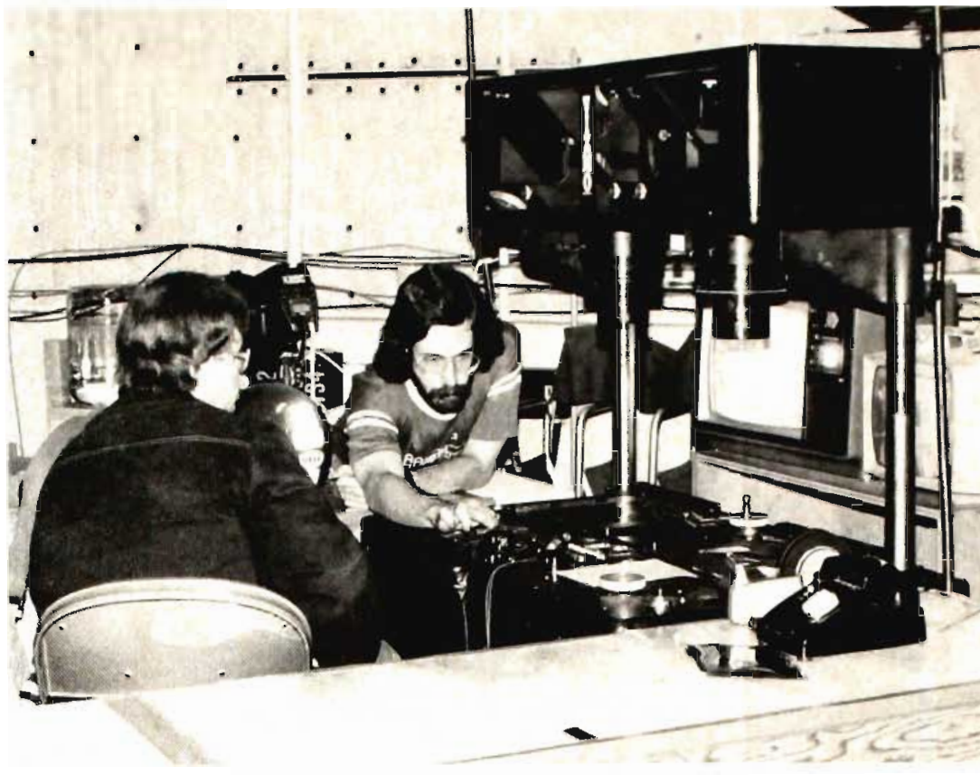
At KNBC-TV, Los Angeles, news graphics are handled by an independent company called "Vizmo", who also handle news graphics for NBC and ABC nightly newscasts. Basically, Vizmo is a rear projection system (similar to an overhead projector, yet much larger and more complex) with super, dissolve, and wipe capabilities. Pictured above is one set of dual Vizmo machines behind the 4' x 5' projection screens on the news set, with author Nick Yermakov, (L), and Vizmo artist, Jim Elyea.
