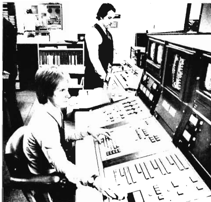
A technician operates Mutual's new computerized master control console. It will enable Mutual to feed up to six network programs simultaneously when combined with the network's planned satellite distribution system.
