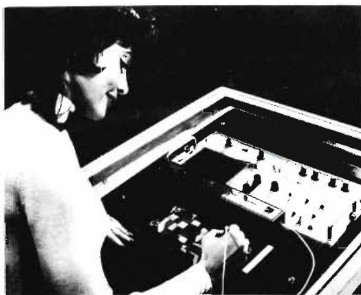
"Telestrator" unit produces hand-drawn or pre-programmed t.v. graphics by simply writing over the video image with an "electronic pen".
