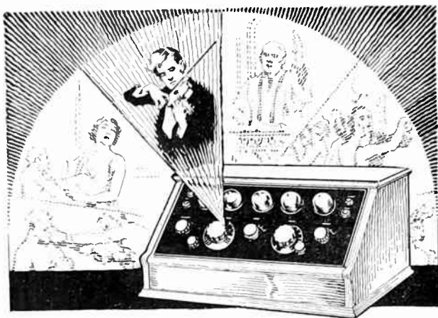
MODEL XV. Two stages tuned R. F. detector and two stages A. F. Simplified tuning on two dials. Stations are always found at the same dial setting. The volume is under control and the tone is musically pure. Retail $142.50 without accessories.
