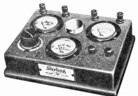
Figure 3. This is the tester commonly used by radio dealers for sales purposes. It requires separate batteries for operation, or independent connections to power supply.
