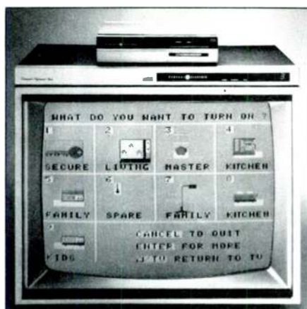
Computers are the catalyst, coordinator, and intersection of the converging media. A set-top computer links television, telephone, and home appliances in the GE HomeMinder system (above).
