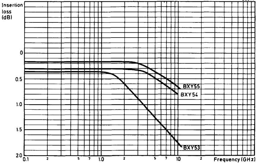
TYPICAL INSERTION LOSS AS A FUNCTION OF FREQUENCY
