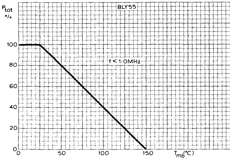
PERCENTAGE POWER DERATING PLOTTED AGAINST MOUNTING-BASE TEMPERATURE FOR FREQUENCIES < 1.0MHz
