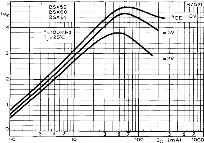
TYPICAL VARIATION OF SMALL SIGNAL FORWARD CURRENT TRANSFER RATIO WITH COLLECTOR CURRENT
