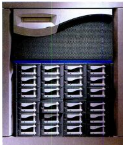
Quantel's sQ server stores each frame of video as a separate entity, not as part of a file.
