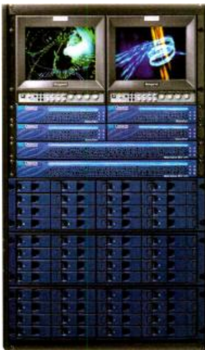
Omneon's MCP 2101 Media Server can have up to 96 channels and 1.8 Gb/s of IP bandwidth.
