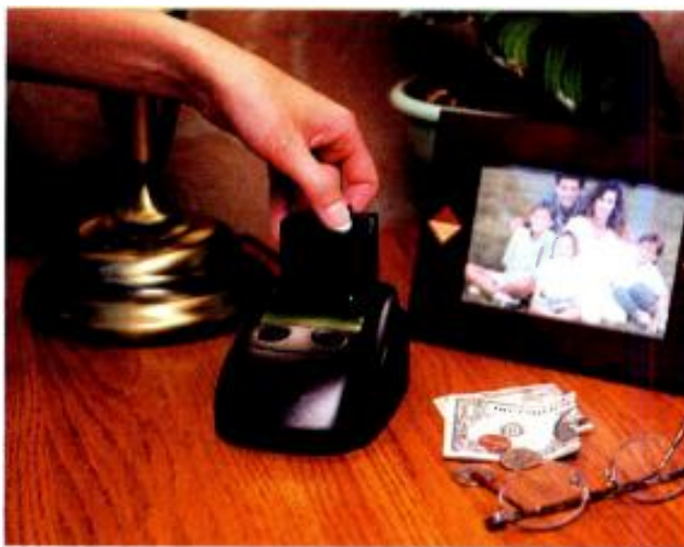
The PPM at rest is still on the job, recording media usage while uploading data to the mother ship at Arbitron.
