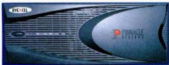
The DVExcell is a frame-based 10-bit DVE that can have as many as 12 DVEs on screen at the same time.
