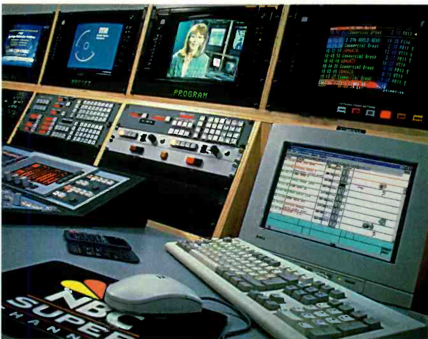
NBC uses Pro-Bel's Automation Internet Schedule Browser, which allows a station-group operator to monitor the activity of individual stations via a WAN.
