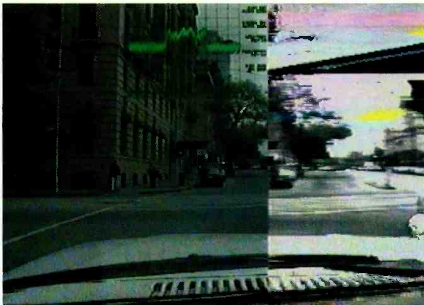
This shot, taken from Tribune's digital ENG trial in Chicago, shows a side-by-side comparison of NDS' digital COFDM system (l) and an analog system (r).
