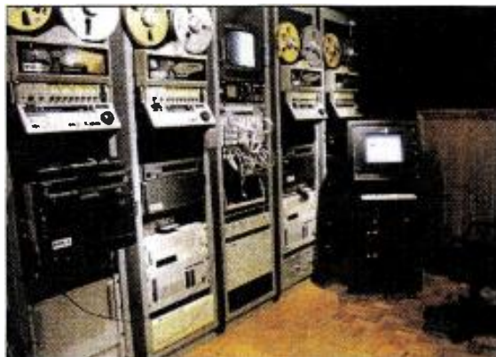
Cyphertech is using its encoding equipment to place digital data in the audio portion of TV programming.
