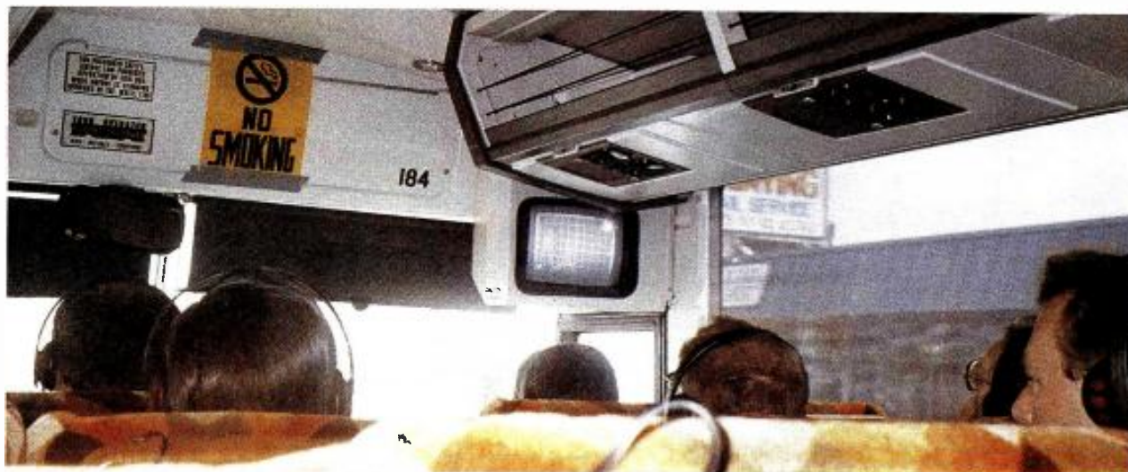
Test monitor on NAB's Eureka 147 demonstration bus suggests multipath impairment. But DAB listeners could not hear it.
