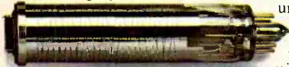
Sony-developed 2/3-inch Mixed Field Saticon. ™ (Plumbicon ™ tubes also available.)
