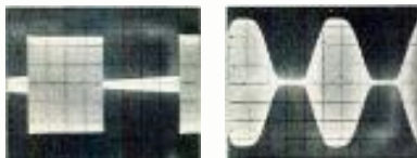
Left: Photo shows excellent dynamic response of Continental's 5 kW AM transmitter at 20Hz modulation. Right: photo of modulation wave form shows effect of Instantaneous Peak Limiter
