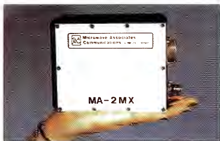
Dimensions: 4 \frac{3}{4} " x 2 \frac{1}{2} " x 5 \frac{3}{4} ", Weight: 3.53 lbs. Power output 12 watts, high stability 21-channel synthesizer, internal VSWR and thermal protection, dual audio channels.
