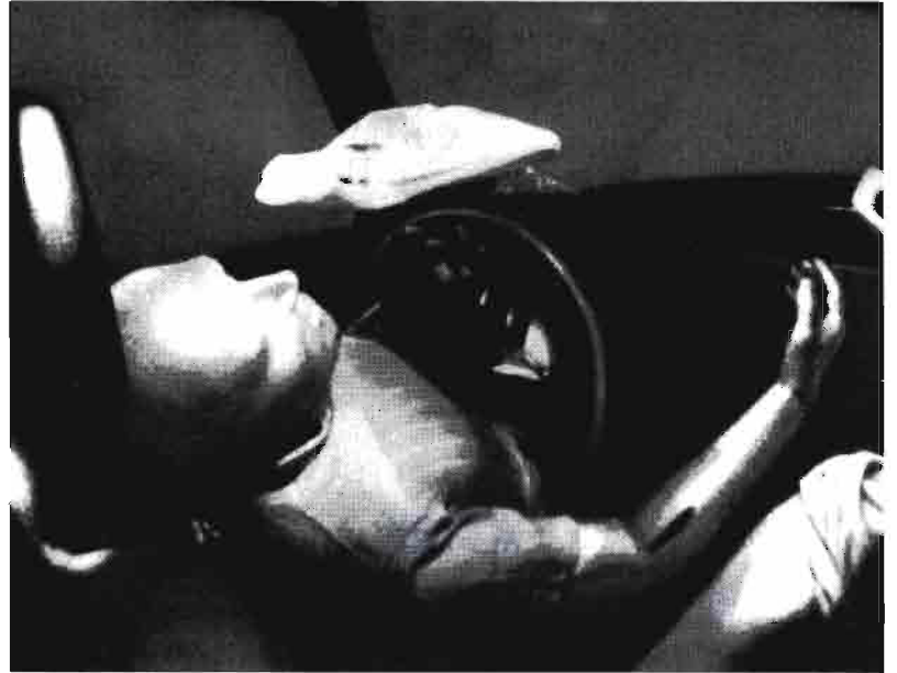
Test dummy, unbelted, in 1975 Volvo sedan without an air bag protection system hitting a test barrier at 35 miles per hour.
