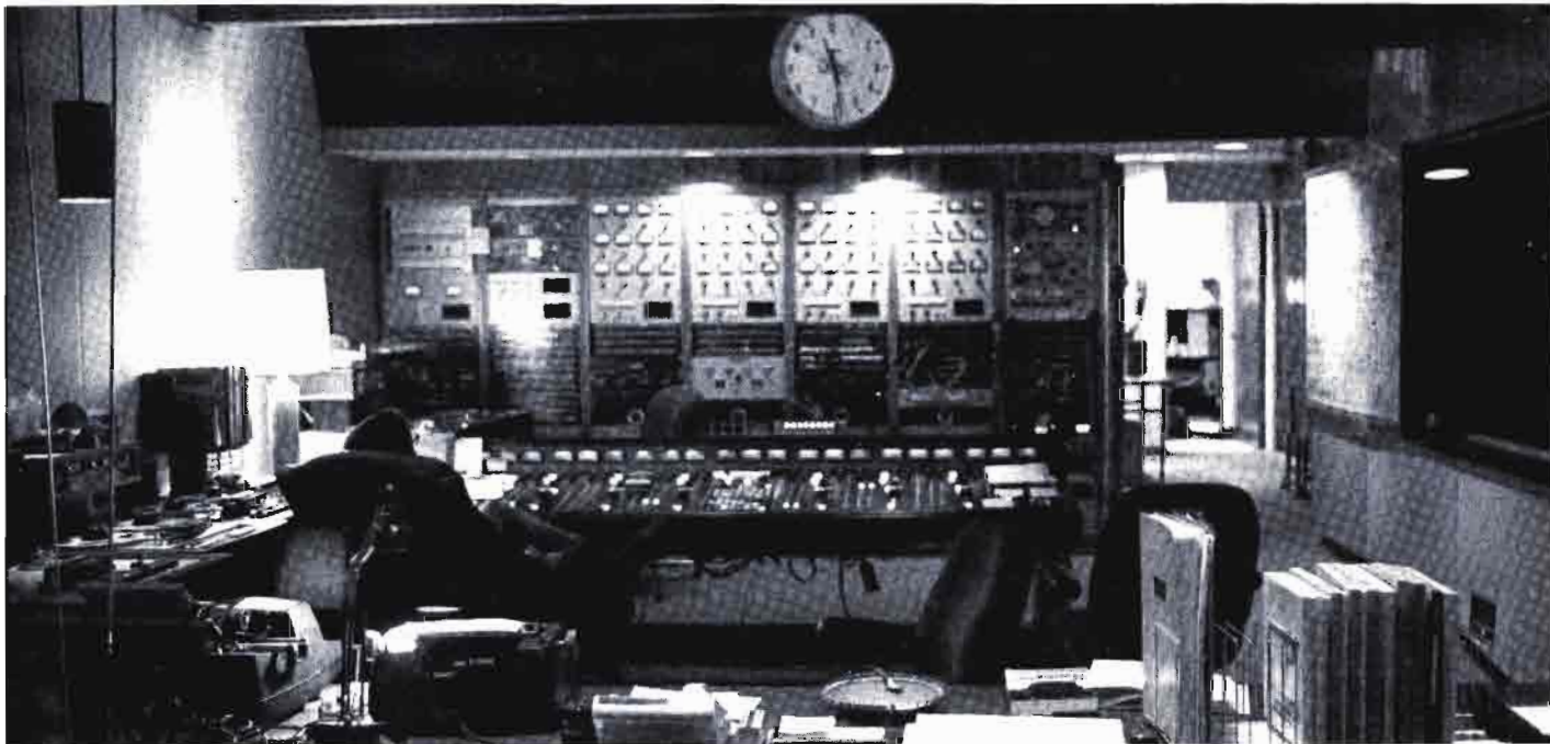
Nerve center. National Public Radio's control room at its Washington headquarters, from which signals are microwaved to the main origination terminal in Bryn Mar, Va. When NPR's satellite system is complete, there will be 17 uplinks nationwide. Seven uplinks are presently operational, and 127 stations are receiving signals from the satellite. Below: All Things Considered co-hosts Susan Stamberg and Sanford Ungar.
