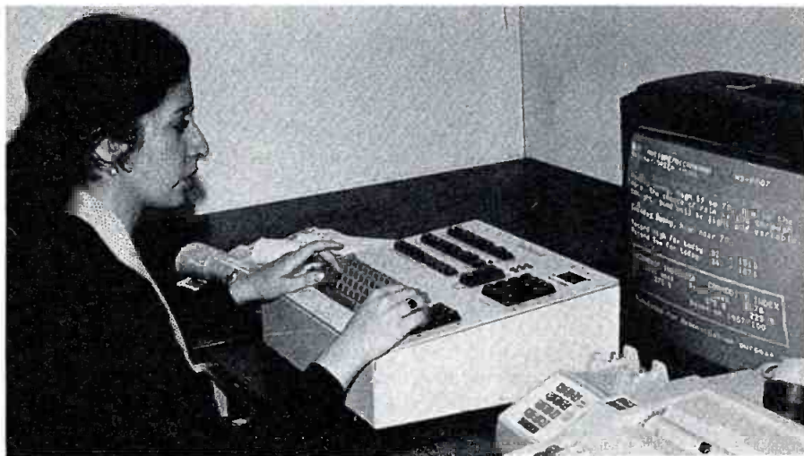
What goes in. Armed with a standard computer terminal and a telephone, a technician programs an Antiope page.
