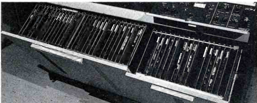
Authors. Maurice Lemoine (l) and Joachim Diermann standing by the experimental digital videotape recorder demonstrated by Ampex during the SMPTE conference in San Francisco Feb. 3. The machine is a modified AVR-3 quadruplex model, reconfigured as an "octoplex"—with eight recording heads—for digital operation. Below. A close-up of the electronics bay.
