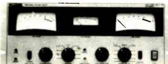
TBM-2200A Stereo Modulation/Frequency Monitor designed to be used in conjunction with the TBM-3500B or TBM-3700.
