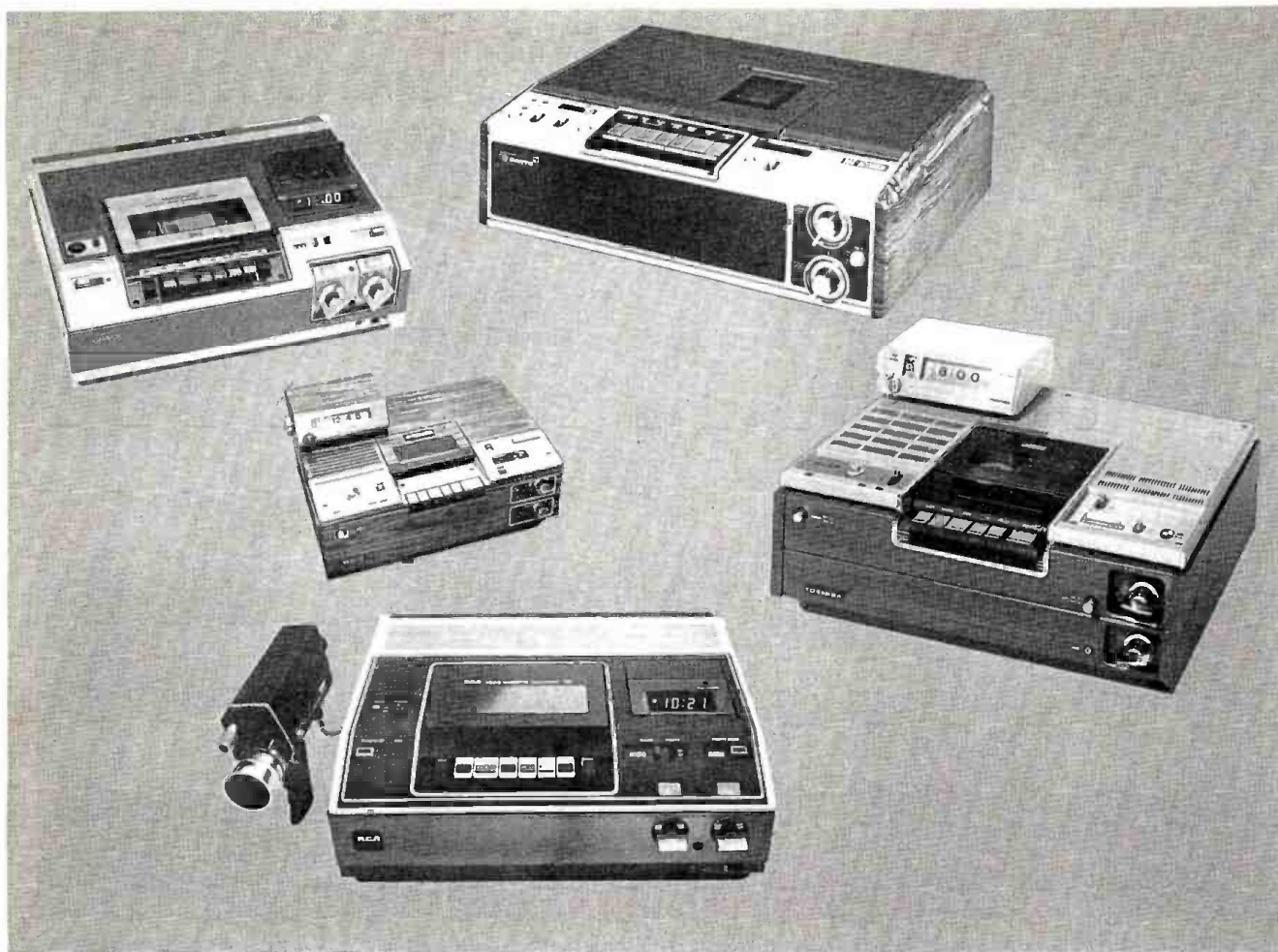
Also running. These five versions of home VTR's—three utilizing Sony's Betamax format (Zenith, Sanyo and Toshiba), two-utilizing the JVC/Matsushita VHS format (RCA and Magnavox)—are prominent in the consumer competition. Sanyo also plans a "V-Card" format model.
