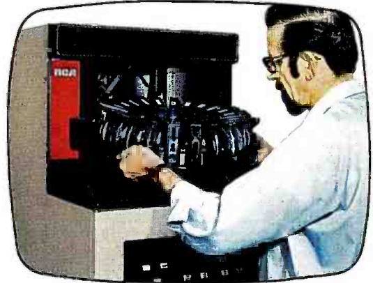
Each cartridge can contain from ten seconds to two minutes of film, with complete cartridge flexibility.
