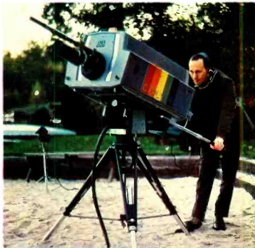
RCA Color Camera set up to test technical capabilities. A Cassegrain type telescope, focal length 125 inches, was installed on the camera to produce the moon-shot shown here.
